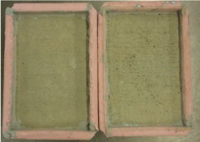
Figure B.1 Appearance of specimens that were subjected to scaling test in the presence of 4% solution of sodium chloride (NaCl) after 100 cycles of exposure (left – Type I; right – FA) sodium chloride with magnesium chloride.
