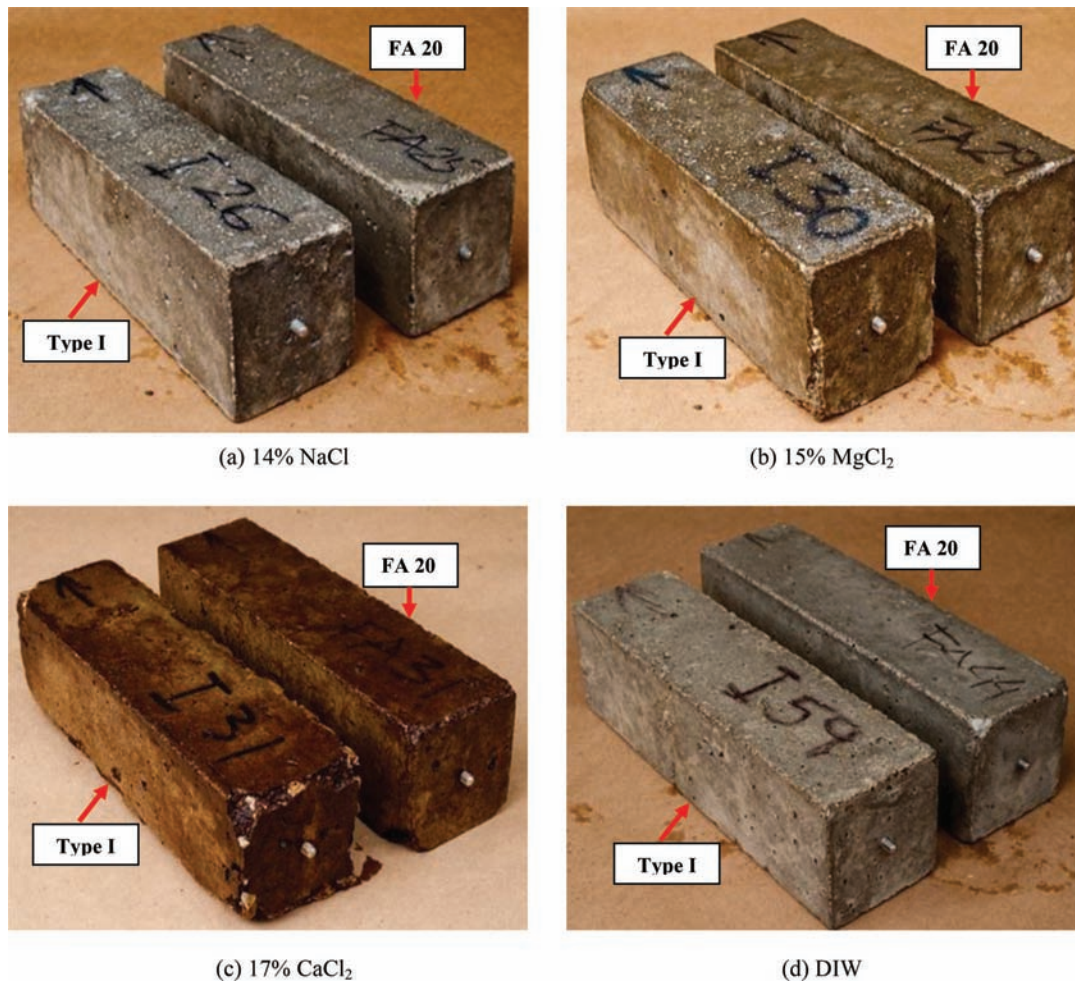
Figure 4.1 Appearance of test specimens subjected to 168 F/T cycles in the presence of three different deicing solutions and the deionized water (DIW).
