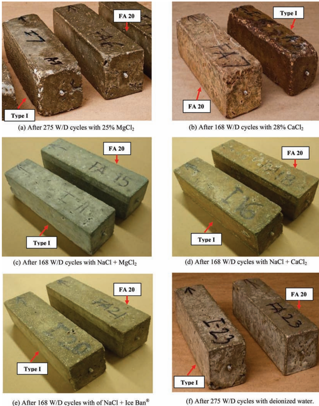
Figure 4.2 Appearance of test specimens subjected to 168 W/D cycles in the presence of different deicers or the deionized water (DIW).
