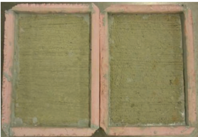
Figure B.2 Appearance of the specimens that were subjected to scaling test in the presence of the combination of sodium chloride with magnesium chloride (NaCl + MgCl 2 ) after 100 cycles of exposure (left – Type I; right – FA).
