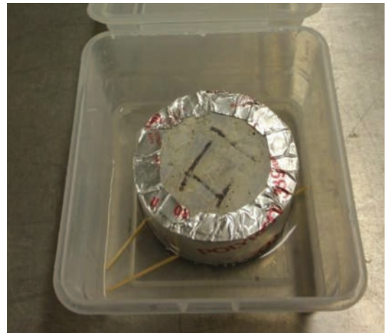
Figure 3.1 Picture of absorption test setup.
