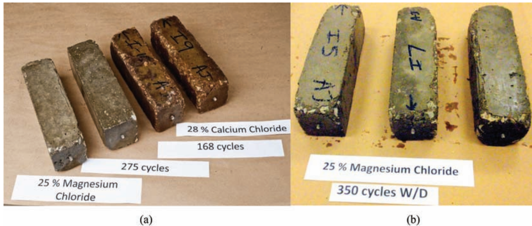
Figure 4.3 Type I specimens subjected to (a) 275 and 168 WD cycles in 25% MgCl 2 and 28% CaCl 2 solutions, and (b) Type I specimens subjected to 350 WD cycles in 25% MgCl 2 .
