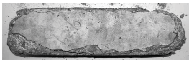
Fig. 10—Specimen subjected to 10 weeks of exposure to 6.04 molal ion concentration solution of MgCl 2 .
