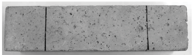
Fig. 3—Specimen subjected to 95 weeks of exposure to distilled water.
