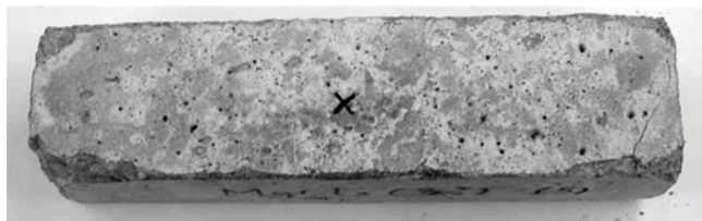
Fig. 6—Specimen subjected to 80 weeks of exposure to 1.06 molal ion concentration solution of MgCl 2 .
