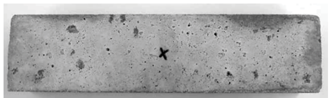
Fig. 4—Specimen subjected to 95 weeks of exposure to 1.06 molal ion concentration solution of NaCl.
